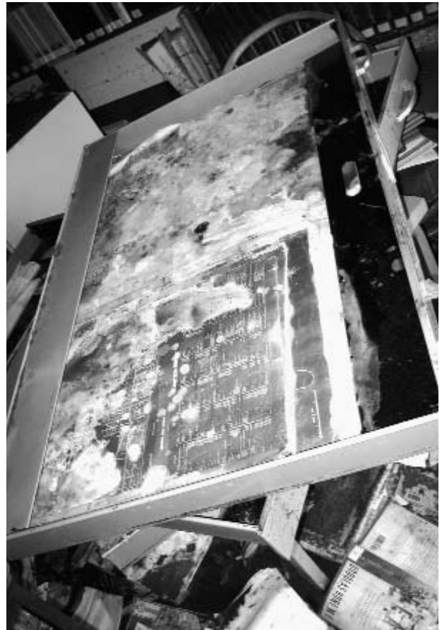
Mold damage inside a map drawer, Biloxi Public Library, Biloxi, Mississippi: 27 September 2005
